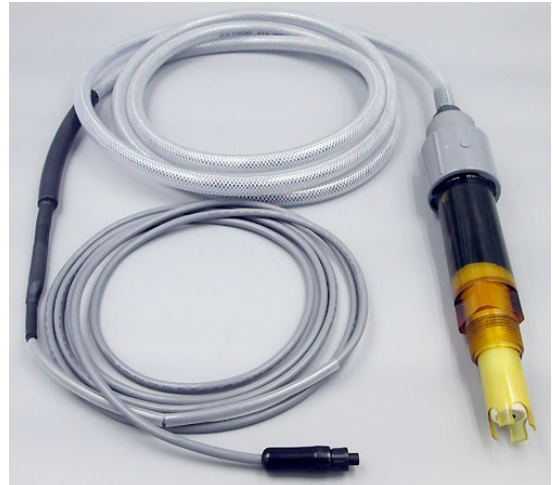
AB 6100 fluoride ion selective submersible sensor with integral preamplifier; WPH waterproofing option & Q7M NEMA6P rated snap connector for use with Q7F-Xm-TL female snap to tinned lead extension cables
