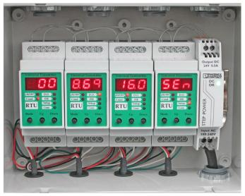
Type of connected sensor is indicated with illuminated LED in main display mode. Additional parameters beyond main process value can be shown using the 'Up' and 'Down' keys as detailed in the documentation. Output is configured in setup LED mode.
