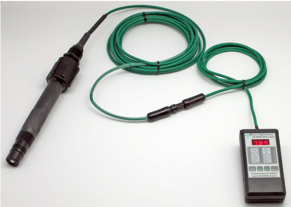
RH-DO-UNIVERSAL-CONVERTIBLE-WPC Smart Digital RS-485 MODBUS RTU dissolved oxygen sensor is ready for immediate field installation into 3/4" FNPT process connection for inline use and 3/4" NPT immersion rod or standpipe for fully submersible use.
