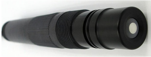
Close-Up on galvanic DO measuring cell of dissolved oxygen sensor in convertible configuration in fully assembled state ready to use.
