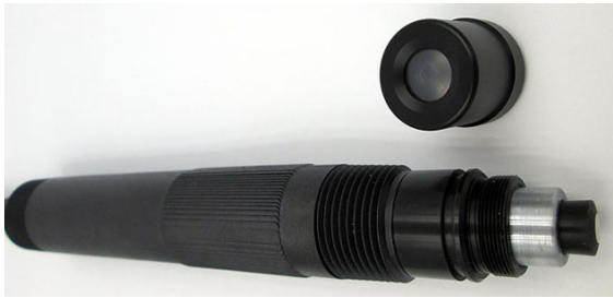
Disassembled galvanic DO measuring cell ready for rebuilding. Cathode & anode on front tip of sensor are shown to the bottom right. High stability thick membrane installed into cap is shown immediately above. Membrane & electrolyte solution are easily replaced in just minutes when required. There is a virtually unlimited sensor lifetime achieved with this rebuildable type galvanic DO cell ensuring a very low total cost of ownership.
